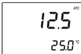
**Note:** The ATC tag blinks and automatic temperature compensation is disabled if the temperature exceeds the 10-40 °C / 50-104 °F range.
