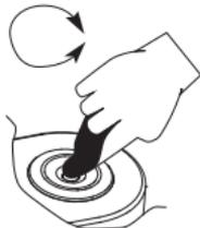
2. Using plastic pipettes, drip sample onto the prism surface. Fill the well completely.
