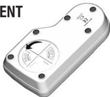
Detach the battery from the terminals and attach a fresh 9V battery while paying attention to the correct polarity. Insert the battery and replace the cover.
